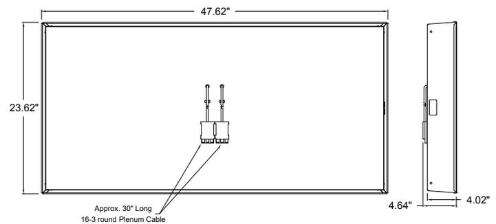
Notes: 1. Dimensions are in inches 2. GPI units are not for use in Plenum ceilings 3. GPI units are built to UL-48 specifications
