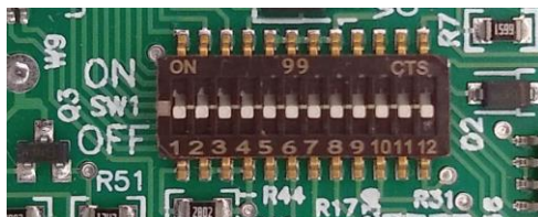
ECL-42-01 Driver setting – all off For use with old ECL-47-00 Active Keypad
