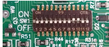
ECL-42-02 Driver setting – just 9 & 10 on For use with new ECL-49-00 Passive Keypad
